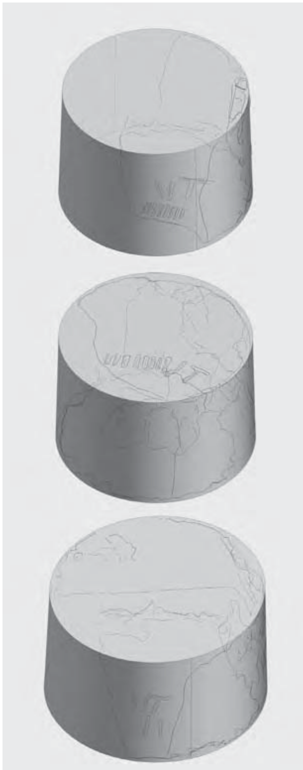
Fig. 3. Axonometric representation of the unprocessed total station data with fitted semi-transparent truncated cones (based on 2008 survey data). By J. Pakkanen.
