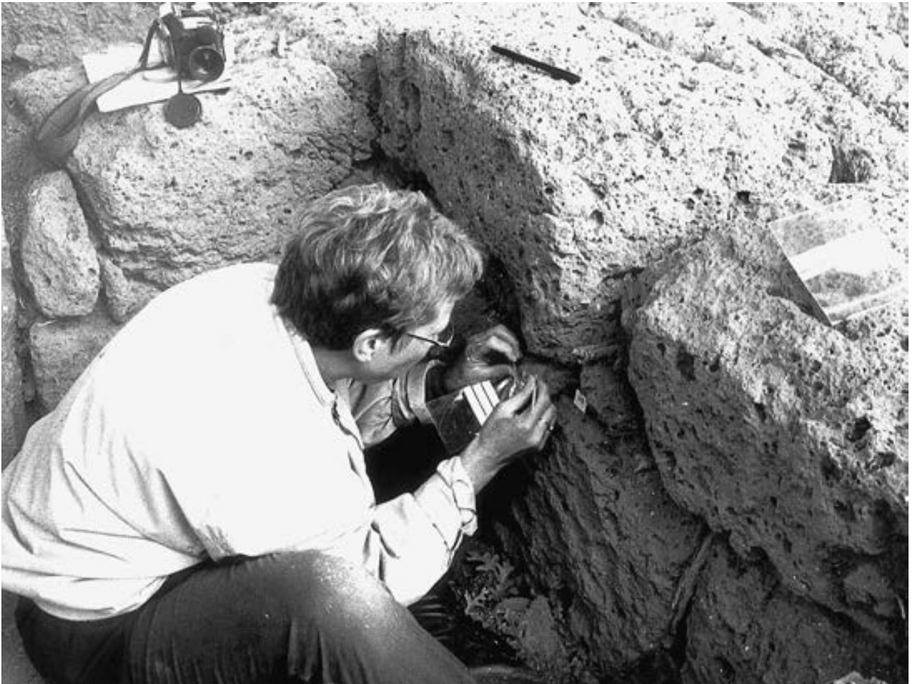
Fig. 141. It was quite difficult to extract a big enough piece to be suitable for analysis, from the frail material in the joints. Photograph by B. Blomé.
