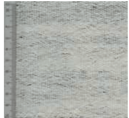
Fig. 4. Example of a weft-faced weave with an average of 5.8 warp and 14.8 weft threads per cm. Courtesy Eva Andersson Strand © CTR.
