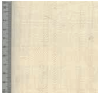
Fig. 3. Example of a 2/2 twill weave with 14.6 warp threads and 14.6 weft threads per cm. Courtesy Eva Andersson Strand © CTR.
